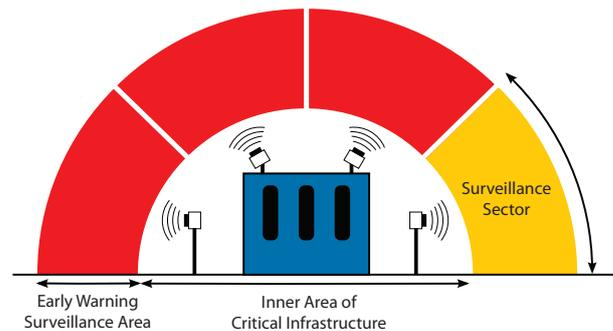
Fig. 1. A model picture of a bubble spanning over the CI. The P5 system monitors the shaded early warning area outside the perimeter of the infrastructure area using a sensor network, where each sensor node covers a surveillance sector.
