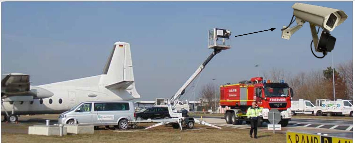
IMST GmbH and the Fraunhofer Institute for Communication, Information Processing and Ergonomics (FKIE) made a radar/video test campaign at the airport Cologne/Bonn. The system controls airport supply vehicle traffic that must cross the aircraft taxiway. If the sensors detect any objects (e.g. suitcases or other goods in transit), persons or vehicles, the intersection will remain closed to aircrafts until the areas has been cleared.
